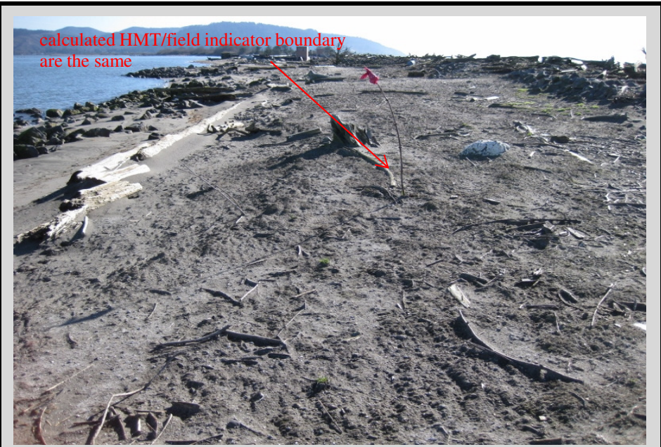
WT-10 E: Calculated HMT and the field indicator boundary are the same.
